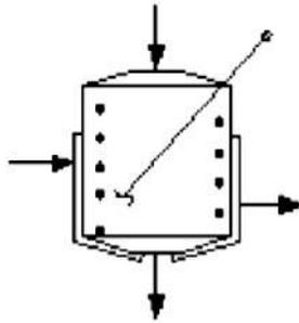
Vessel with Jacket Coil Agitator
