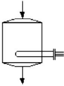
Vessel with Immersion Heater
