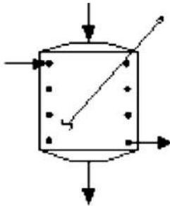
Vessel with Coil and Agitator
