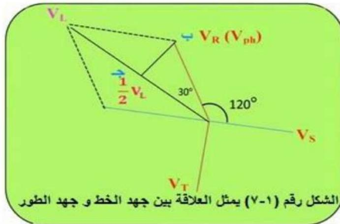
$$\cos 30^\circ = \frac{\frac{1}{2} V_L}{V_{ph}}$$
