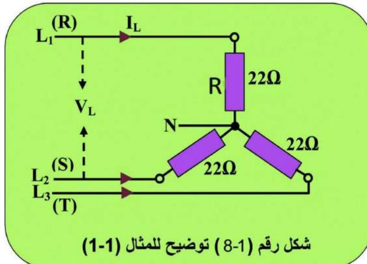
$$V_{ph} = \frac{V_L}{\sqrt{3}} = \frac{380}{1.7} = 220 \text{ V}$$
